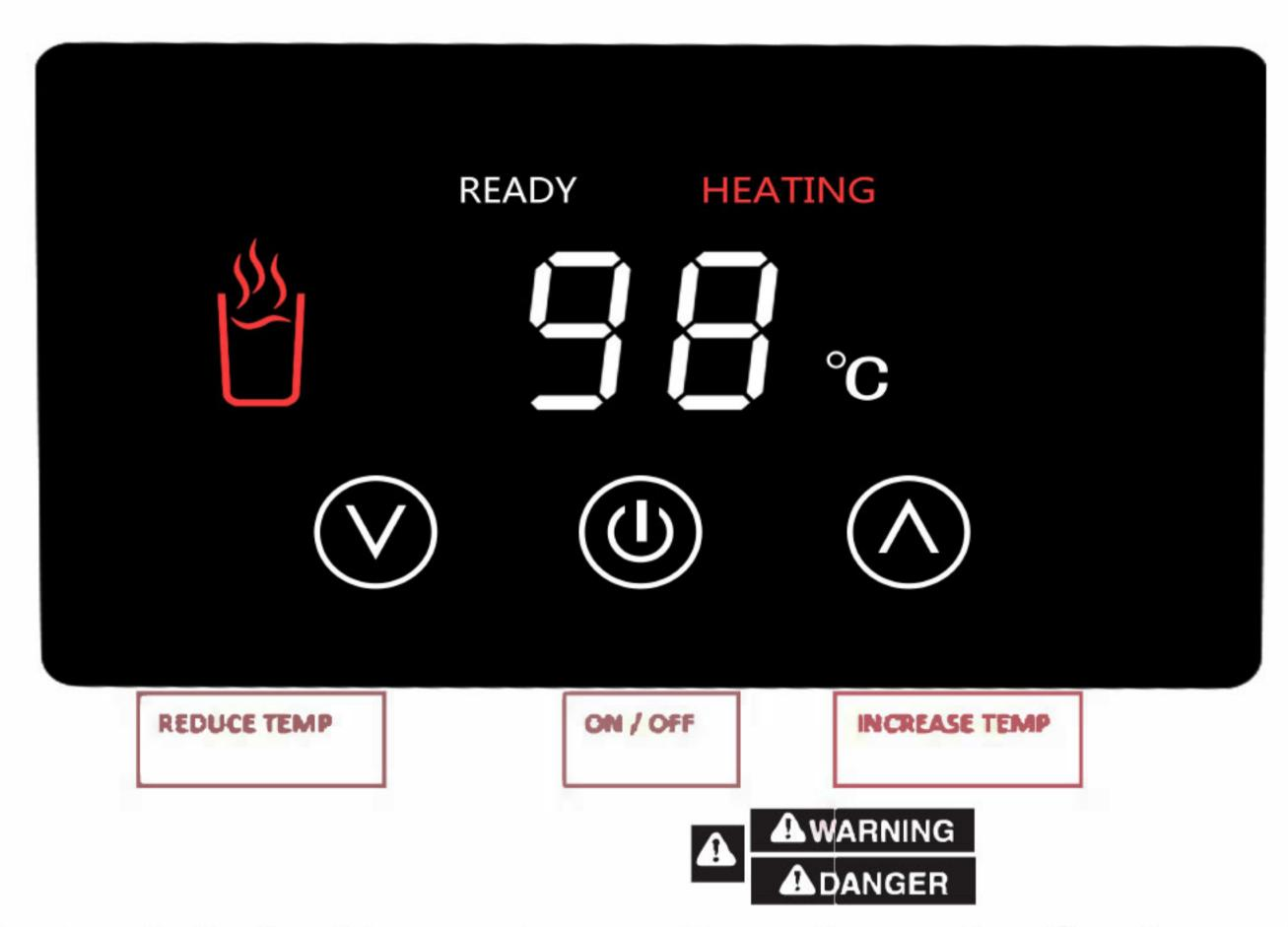
If the electronic instant hot water appliance is empty of water and is turned ON then this will be automatically sensed, the heating element will not energise and the "lack of water" indictor will be flashing on the display panel shown by the flashing of the E3
